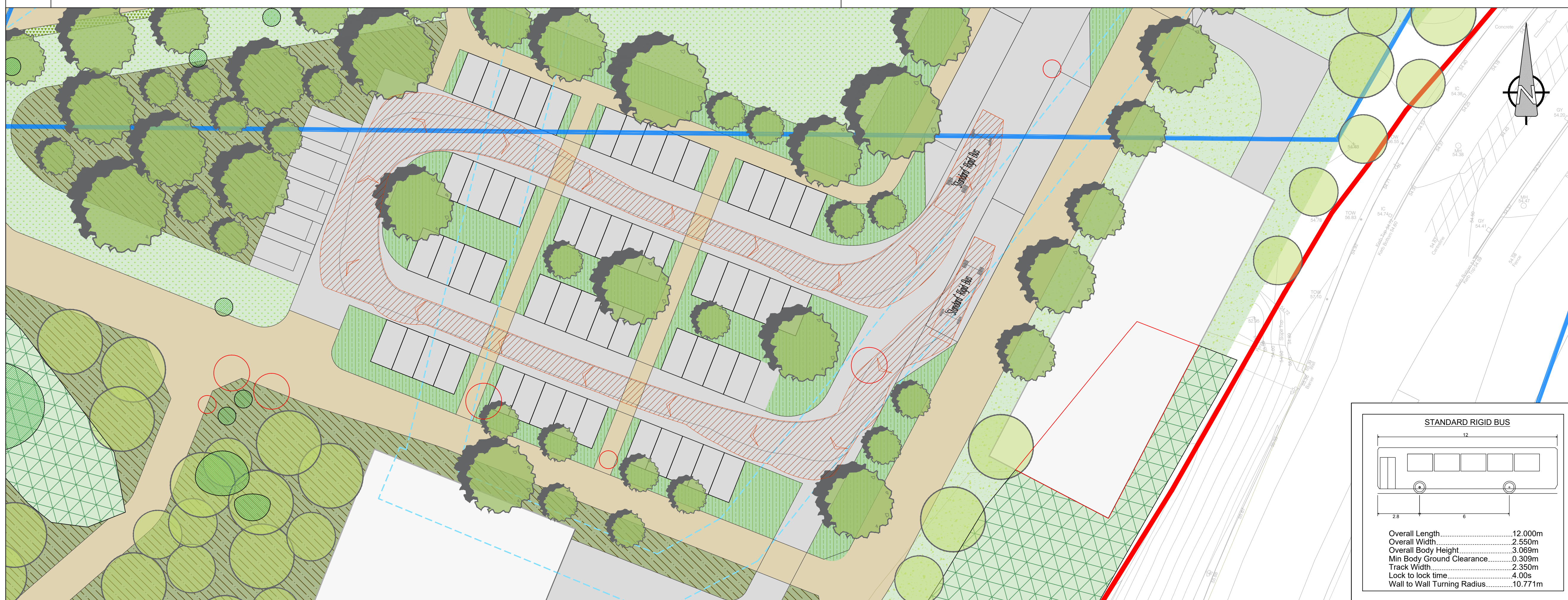
C PROPOSED SWEEP PATH ANALYSIS - BUS 0103 Scale: 1:250
