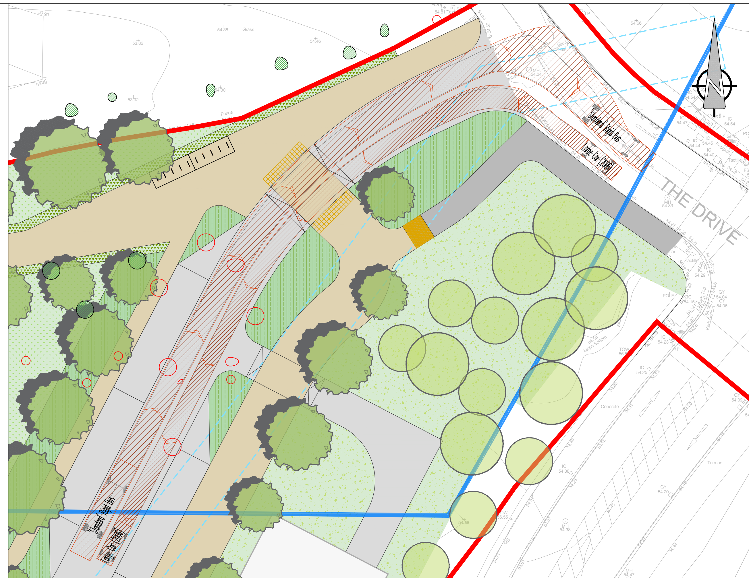
B PROPOSED SWEEP PATH ANALYSIS - BUS EXITING 0102 Scale: 1:250
